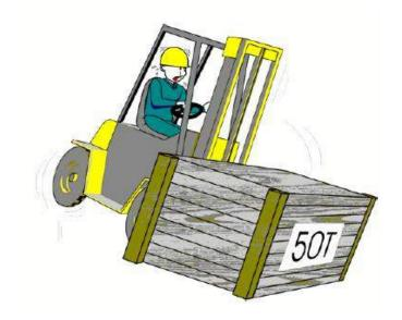
It shall have beeper light and alarm (when reversing); blinking light and seat belt. 义车上应当安装有警示灯和警示笛(倒车时用)和安全带。
